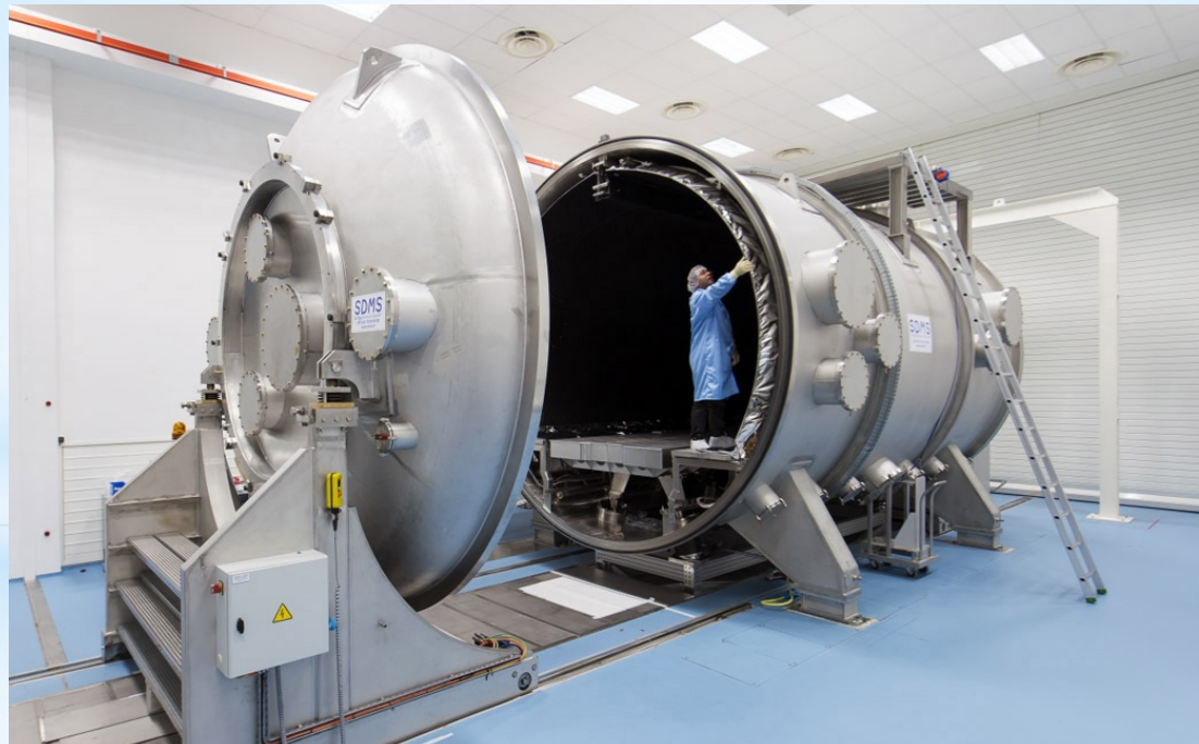
45 m 3 crio-vacuum chamber 77K and 10 -6 mbar
