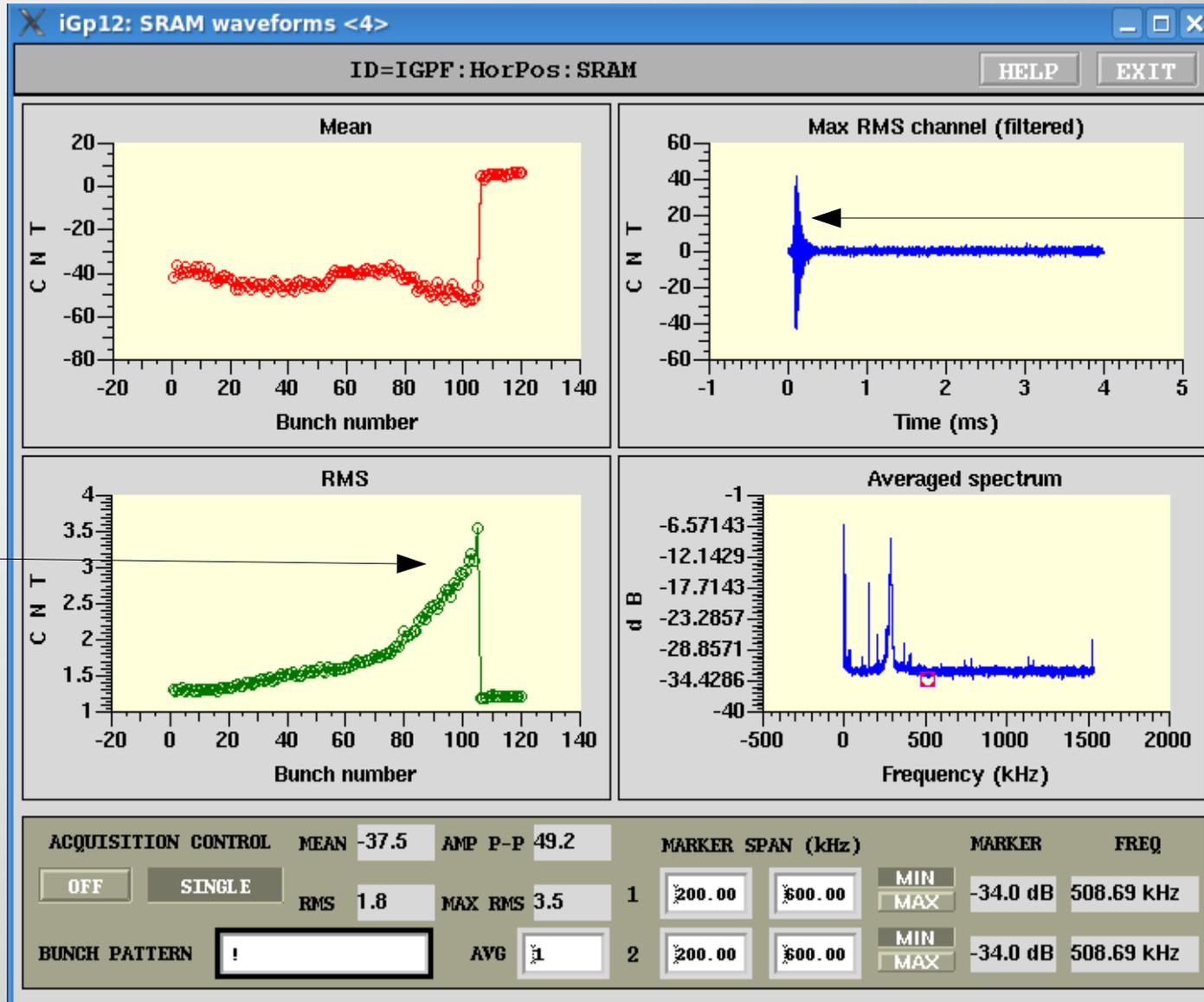
After recording oscillation data during growth and damping period, a modal analysis has been made showing the instability growth rate and the damping feedback performance
