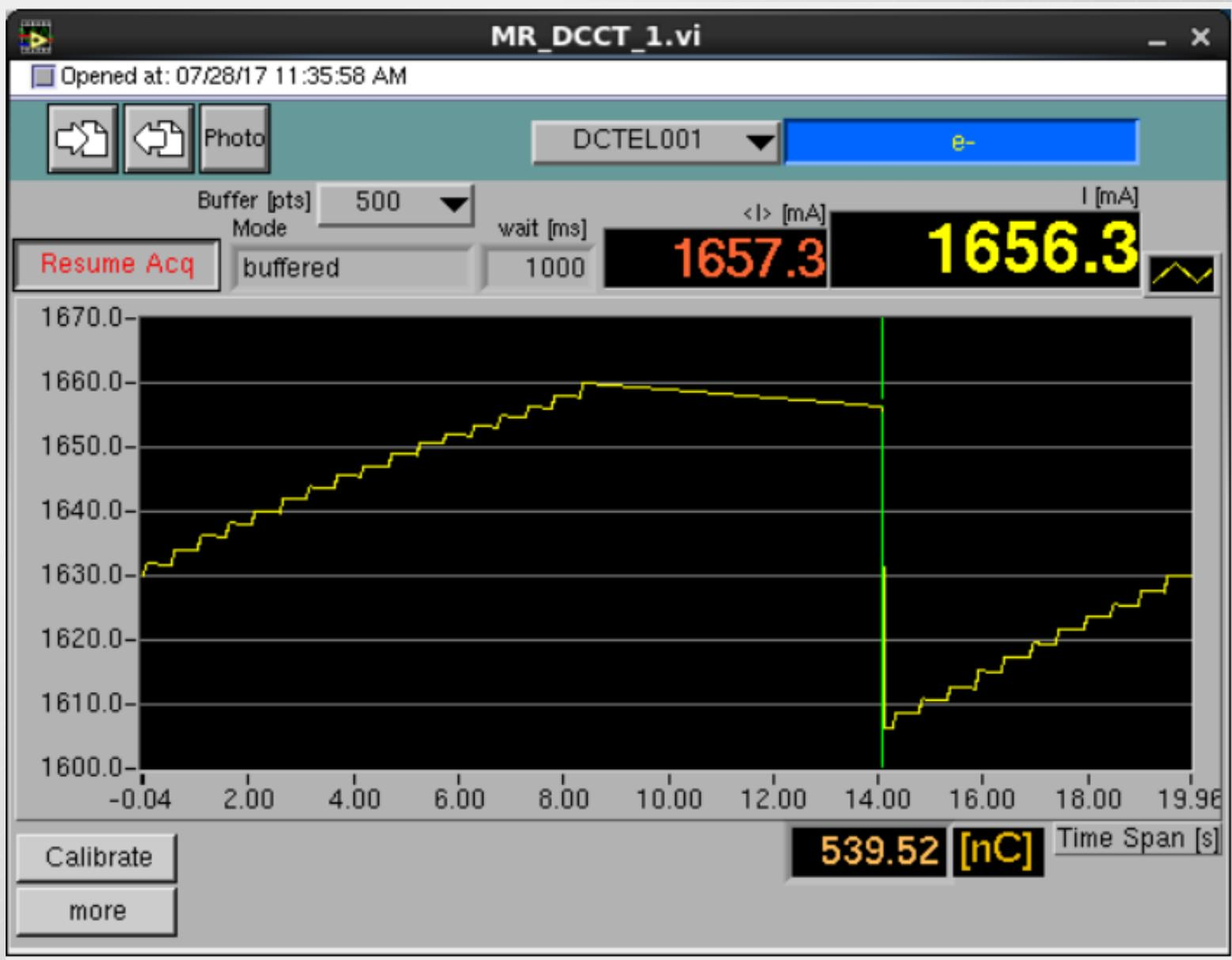
On October 25<sup>th</sup> tests on the positron current limit have been carried on. As shown below a strong, destructive (even if expected) horizontal instability has been observed with beam current > 800mA
