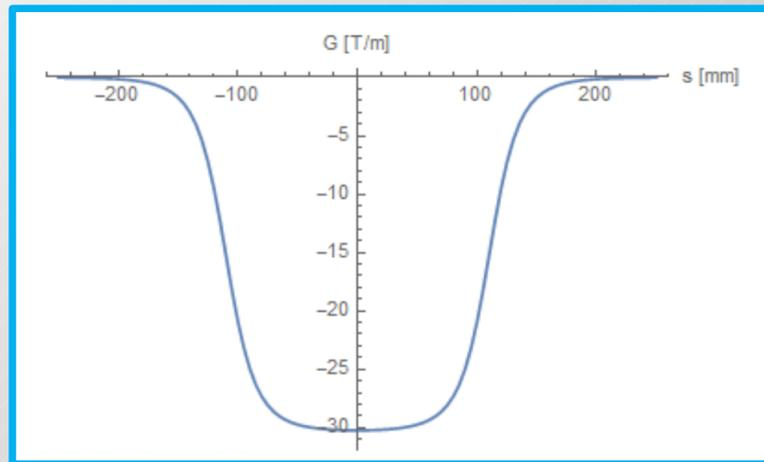
PMQD: longitudinal profile of the field gradient
