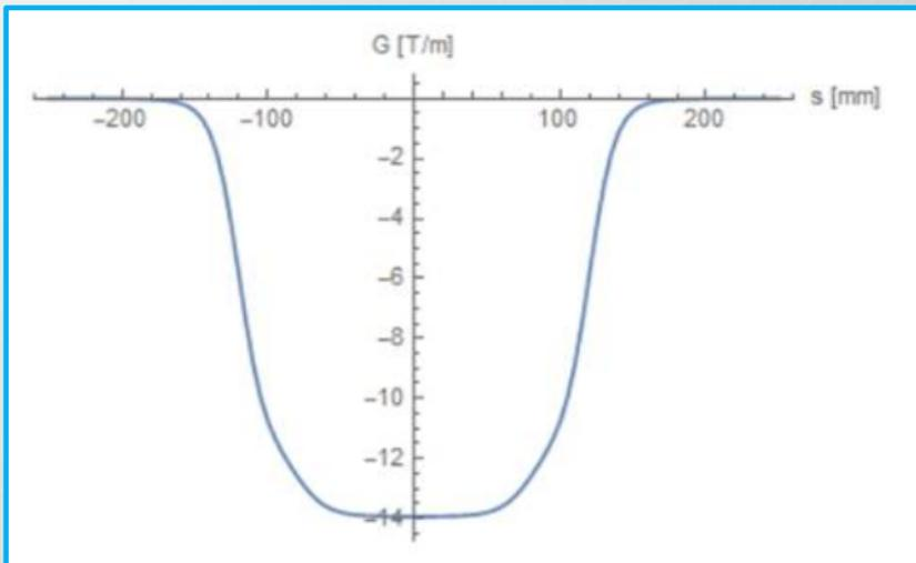
PMQF: longitudinal profile of the field gradient
