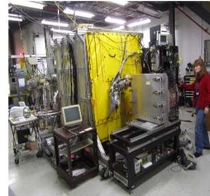
MTAS final design: 19 hexagonal modules, with a central module having a 2.5" hole to accommodate a beam line and auxiliary beta detectors. Each module is 21" long, 8" diameter (6.9" face-to-face) and has custom made carbon fiber housing. Weight ~120 lbs/module, ~2200 lbs total.
