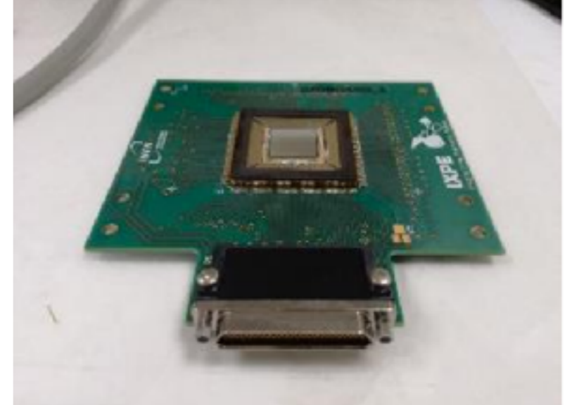
INFN mechanics and PCB, integration with ASIC
