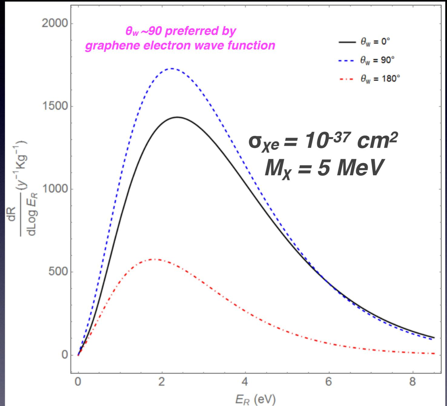
Emission rate from a CNT target at different angles  $\theta_w$
