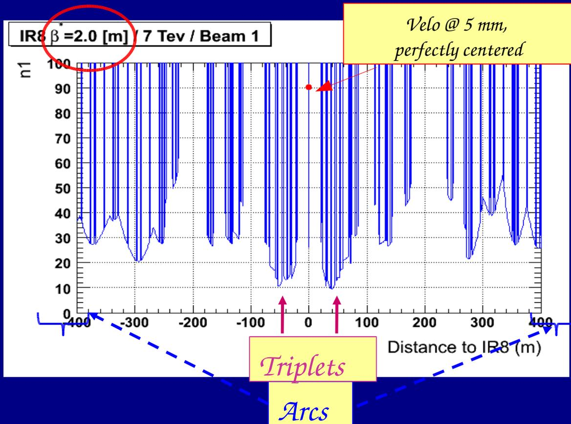
At 5 mm from the beam, VELO remains behind the triplet aperture.
