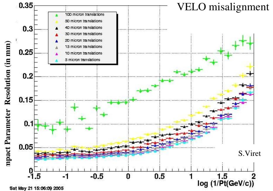
Impact parameter resolution unchanged up to 50  $\mu\text{m}$  shifts
