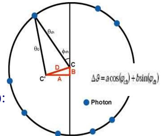
❖ A plot of theta vs phi can be used to extract misalignment parameters.
