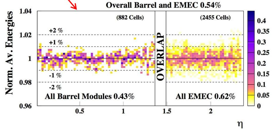
Electron Energy resolution measured in beam tests of the ATLAS EM accordion calorimeter (Pb/LAr)
