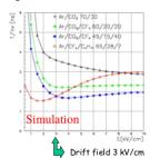
The Ar/CO2/CF4 45/15/40 gas mixture should give the same time performance as the Ar/CO<sub>2</sub>/C<sub>4</sub>H<sub>10</sub> 65/28/7.
