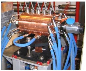
The beam is **streaked** by a **transverse RF cavity** on a **screen**. The image is captured by a camera. Longitudinal charge distribution and centroid position can be measured.
