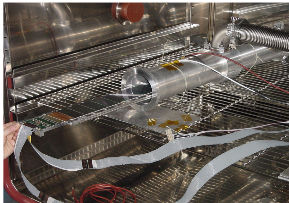
still functioning after -30^{\circ} +60^{\circ} C temperature cycles
