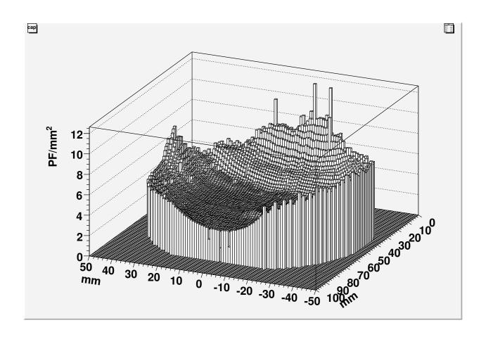
Capacitance [C] distribution.  $\langle C \rangle = 2.8 \text{ pF/mm}^2, \text{ FWHM} = 3.4 \text{ pF/mm}^2.$
