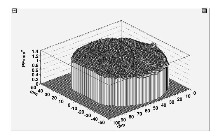
Capacitance [C] distribution. <C> = 1.1 pF/mm<sup>2</sup>, FWHM = 0.34 pF/mm<sup>2</sup>.
