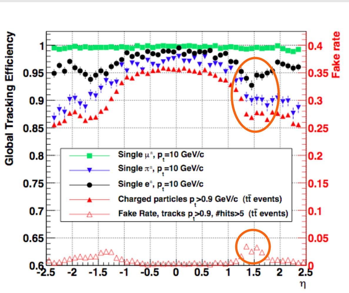
Slight degradation of tracking performances in the transition region between barrel and endcap.
