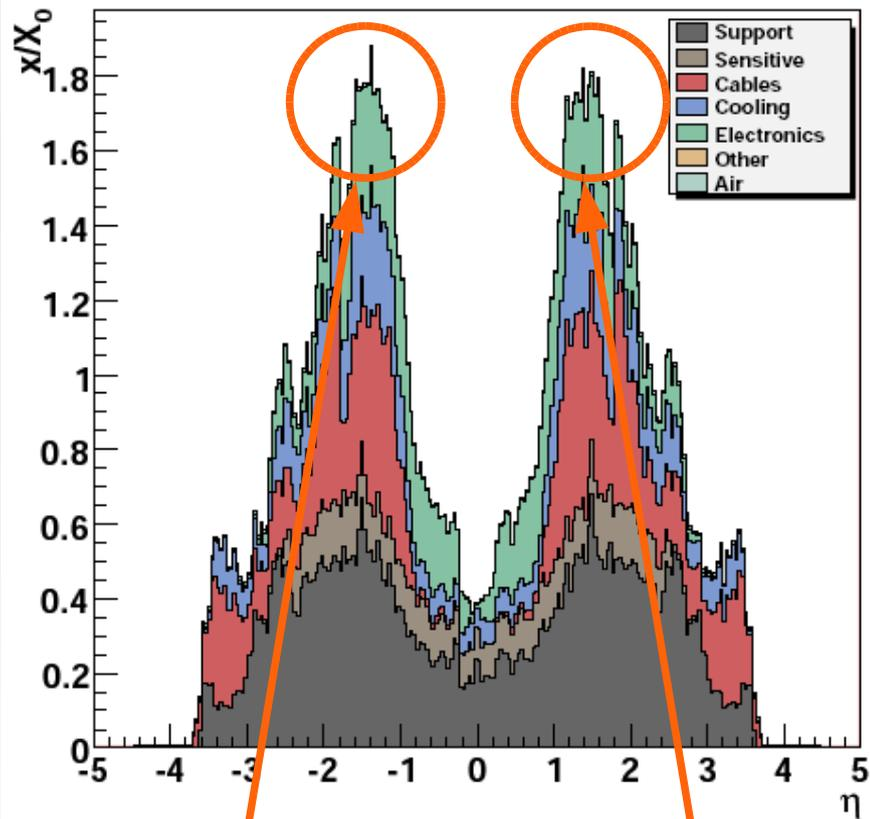
Radiation length up to 1.8 in the transition region barrel-endcap
