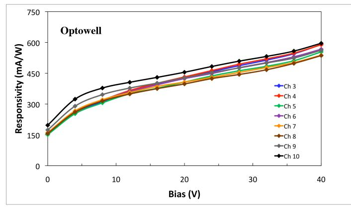
can fully recover pre-irradiation responsivity with high bias voltage
