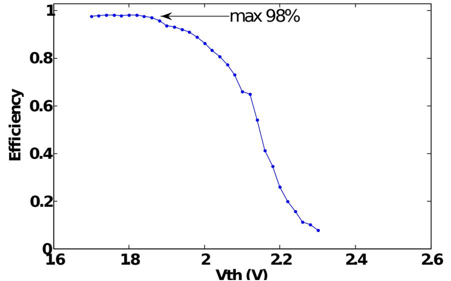
Efficiency remains at 98% for about 150mV above the noise limit.
