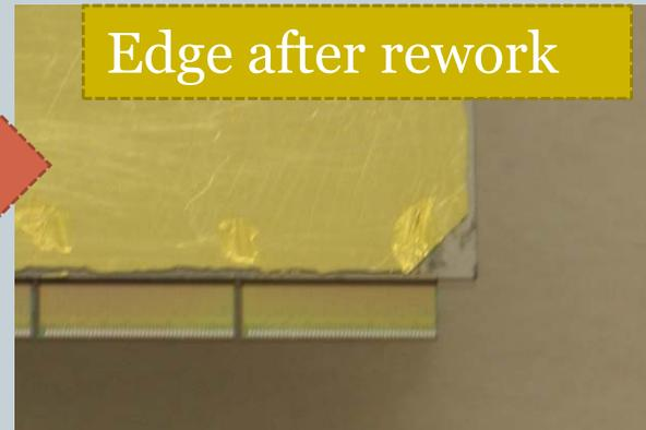
Successful rebuild -> recycling diamond sensors works
