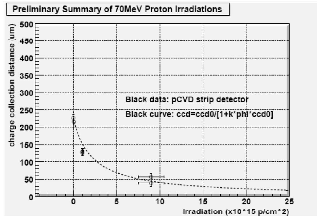
In diamond 70MeV protons have  $\sim 3x$  larger damage constant than 24GeV
