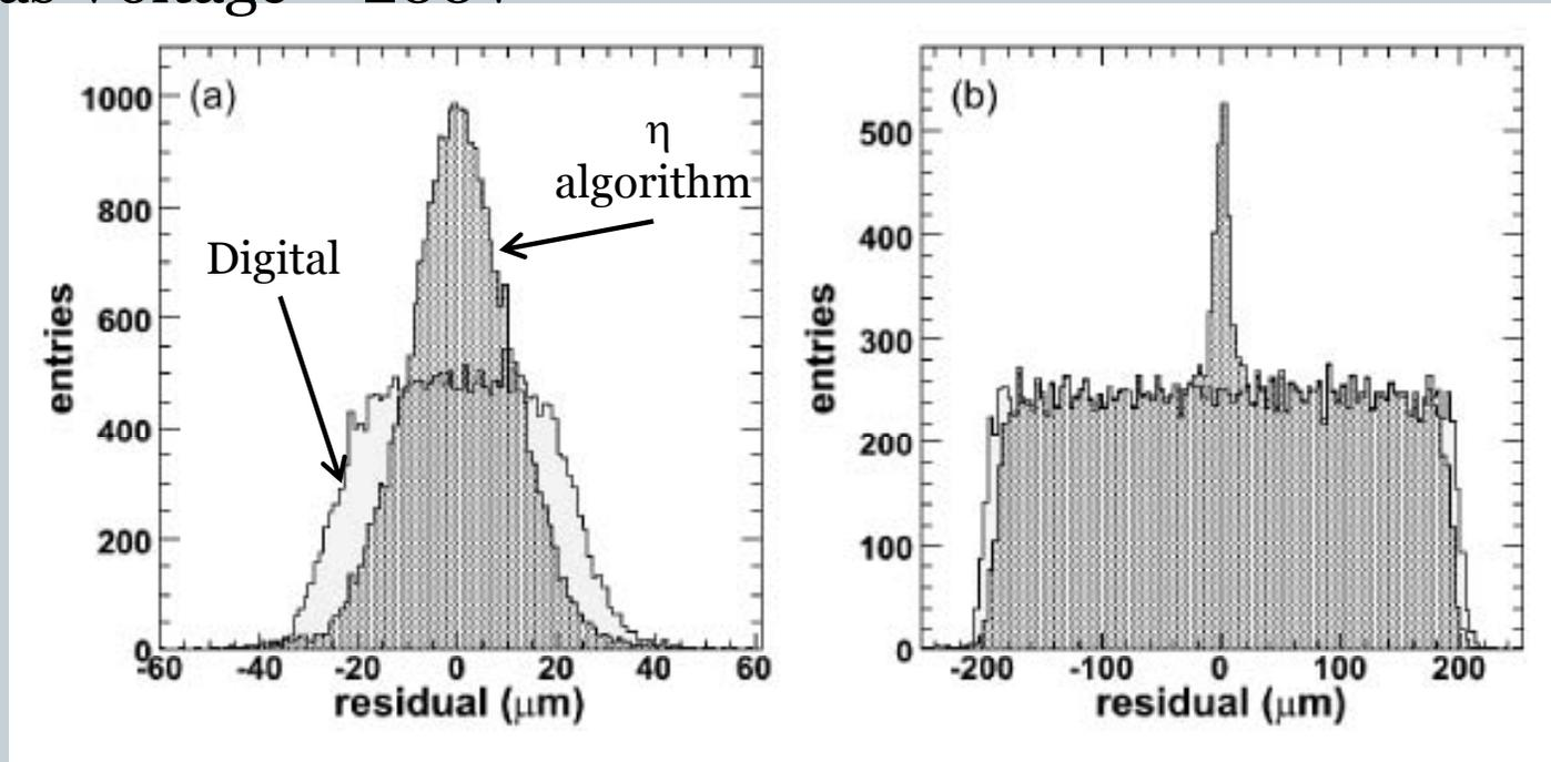
**Measured resolution =  $8.9 \mu\text{m} \pm 0.1 \mu\text{m}$**
