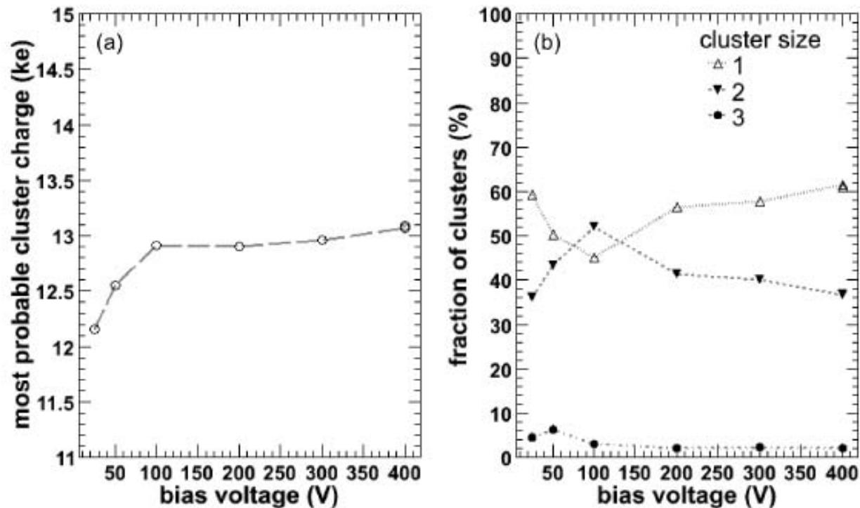
Fig. 5. Most probable values of the charge distribution (a) and fractions of charge cluster sizes (b) as a function of the bias voltage.
