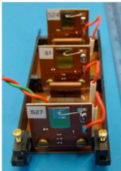
assembled telescope in the cartridge
