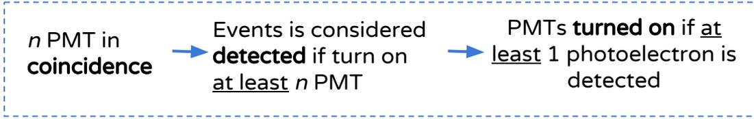
Simulating broken PMTs:
