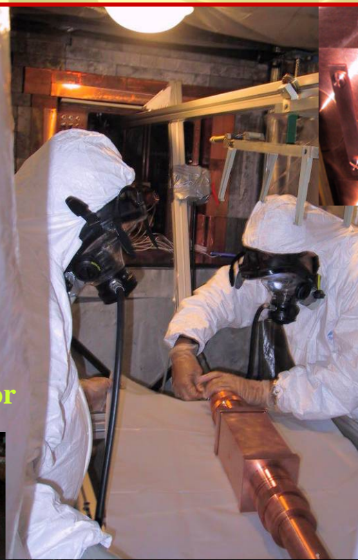
filling the inner Cu box with further shield
