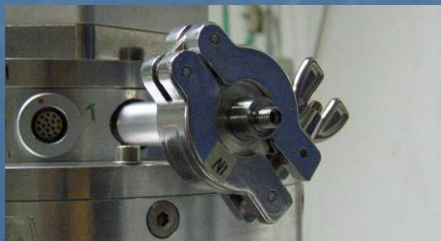
Cryostat modified to have RF ports
