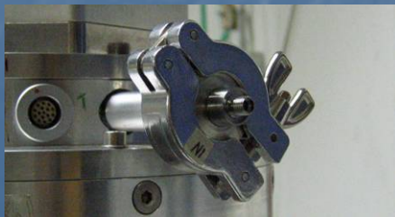
Cryostat modified to have RF ports
