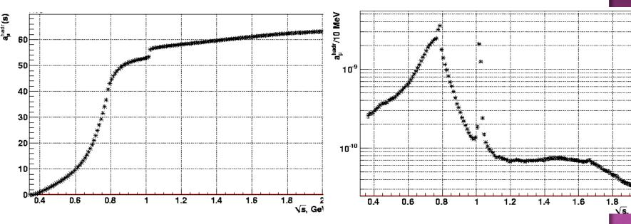
This plot demonstrates how fast integral reaches its asymptotic value  $\sim 60$  ppm. For  $\sqrt{s} > 2$  GeV the contribution is about  $\sim 6$  ppm only
