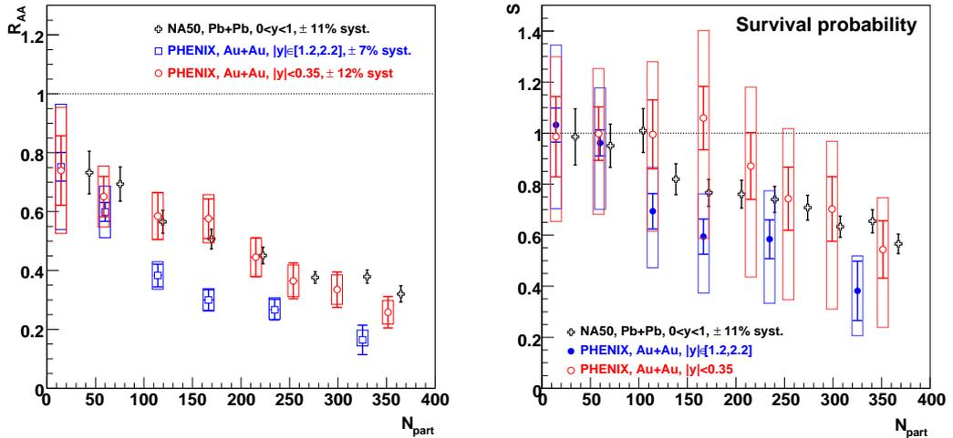
Figure 4:  $J/\psi$  suppression measured by the PHENIX and NA50 experiments, as a function of centrality, given by the number of participants. Left: nuclear modification factor. Right:  $J/\psi$  survival probabilities after normal nuclear effects subtraction.
