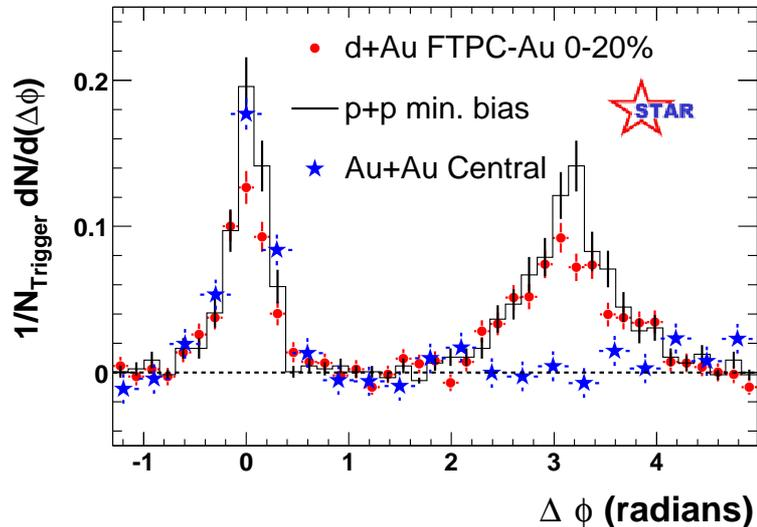
Figure 3: Dihadron azimuthal correlations in p+p, d+Au and Au+Au central collisions, from the STAR experiment.
