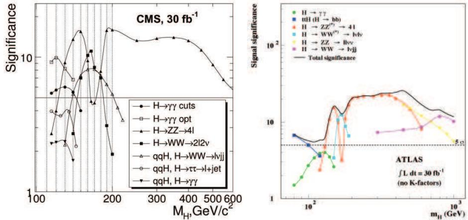
Figure 3: The signal significance as a function of the Higgs Boson mass for  $30 \text{ fb}^{-1}$  of the integrated luminosity for the different Higgs Boson production and decay channels. Analysis results from CMS [9] (left) and ATLAS [10] (right).
