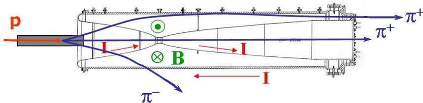
Figure 1: A schematic diagram showing the focusing (de-focusing) of secondary  $\pi^+$  ( $\pi^-$ ) by the magnetic field in between the inner and outer conductors of a neutrino horn (in this case MINOS horn 1).
