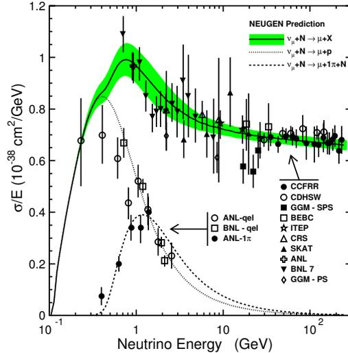
Figure 2: Neutrino cross-section data [14] compared to the prediction from the Neugen program [15]. The dotted curve indicates the quasi-elastic ( $\nu_\mu + n \rightarrow \mu^- + p$ ) contribution and the dashed curve indicates the resonance contribution with a single pion in the final state, (*e.g.*  $\nu_\mu + n \rightarrow \mu^- + \Delta^+ \rightarrow \mu^- + \pi^+ + n$ ) contribution. At higher energies deep inelastic scattering dominates. Plot taken from [16].
