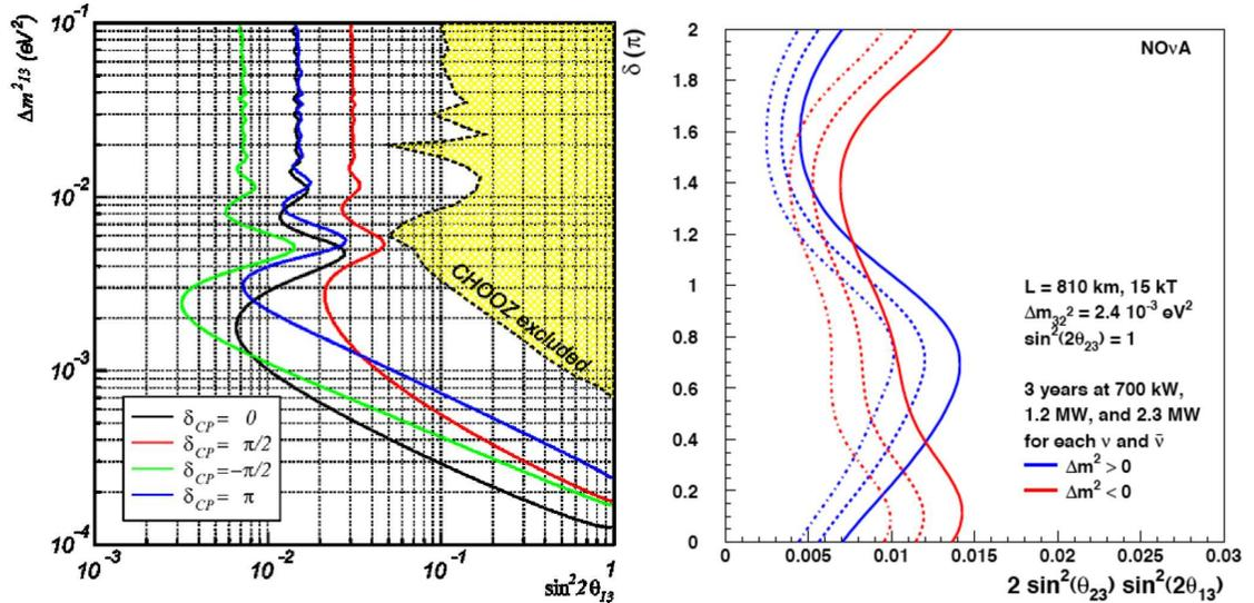
Figure 6: **a)** The expected T2K sensitivity to  $\sin^2 2\theta_{13}$  assuming the nominal Phase I run of 5 years at 0.75 MW. The plot is shown for four values of  $\delta$ . **b)** The expected NO $\nu$ A sensitivity to  $\sin^2 2\theta_{13}$  shown as a function of  $\delta$  and mass hierarchy. Taken from [25].
