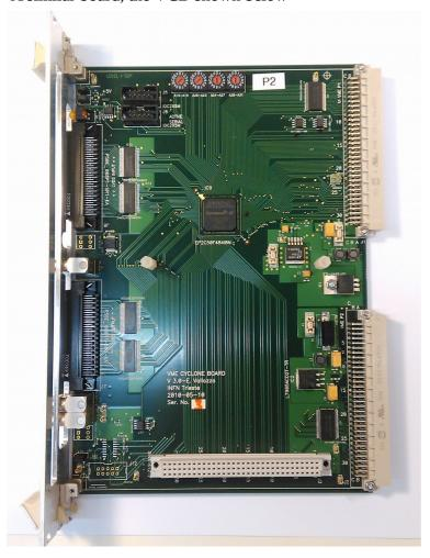
Is equipped with a DIN connector similar to the one on the ADC.
