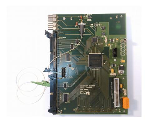
but the communication via the fiber optic cable was asymmetric (only reception). A new board with full-duplex capability could be used on either side of the link. Moreover, modern FPGAs (Altera Cyclone IV and V) provide integrated gigabit links easily interfaced to the fiber optic cables. The board on the VME side would also perform the zero suppression and storage of the data during the spill.
