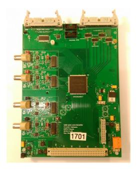
The ADC board is able to read out up to 2 X-Y silicon detector systems (in 2017 we used 1 ADC per detector system). At the moment the two top IDC connectors are used for input and output. All the digital signals from the ADC can also be sent to the DIN connector.
