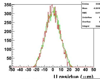
Residual comparison ( data versus GEANT simulation) in the 5 tracking planes in u coordinate
