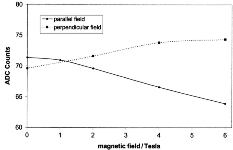
Most probable pulse height of the central pixel as function of the magnetic field parallel and perpendicular to the surface of MIMOSA.
