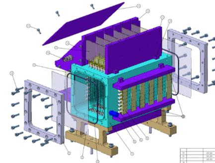
Figure 14 – Tecnical drawing of the BM drift chamber.
