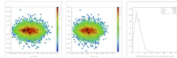
Figure 17 – Beam profile in the two M28 sensors (left and center panel; axis in  $\mu\text{m}$ ). Right panel: reconstructed angular divergence of the beam in mrad.
