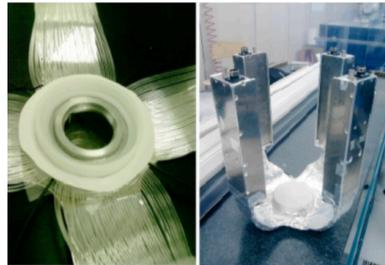
Figure 13 – Details of the Start Counter: the thin scintillator foil and the optical bers grouped in four di erent arms.
