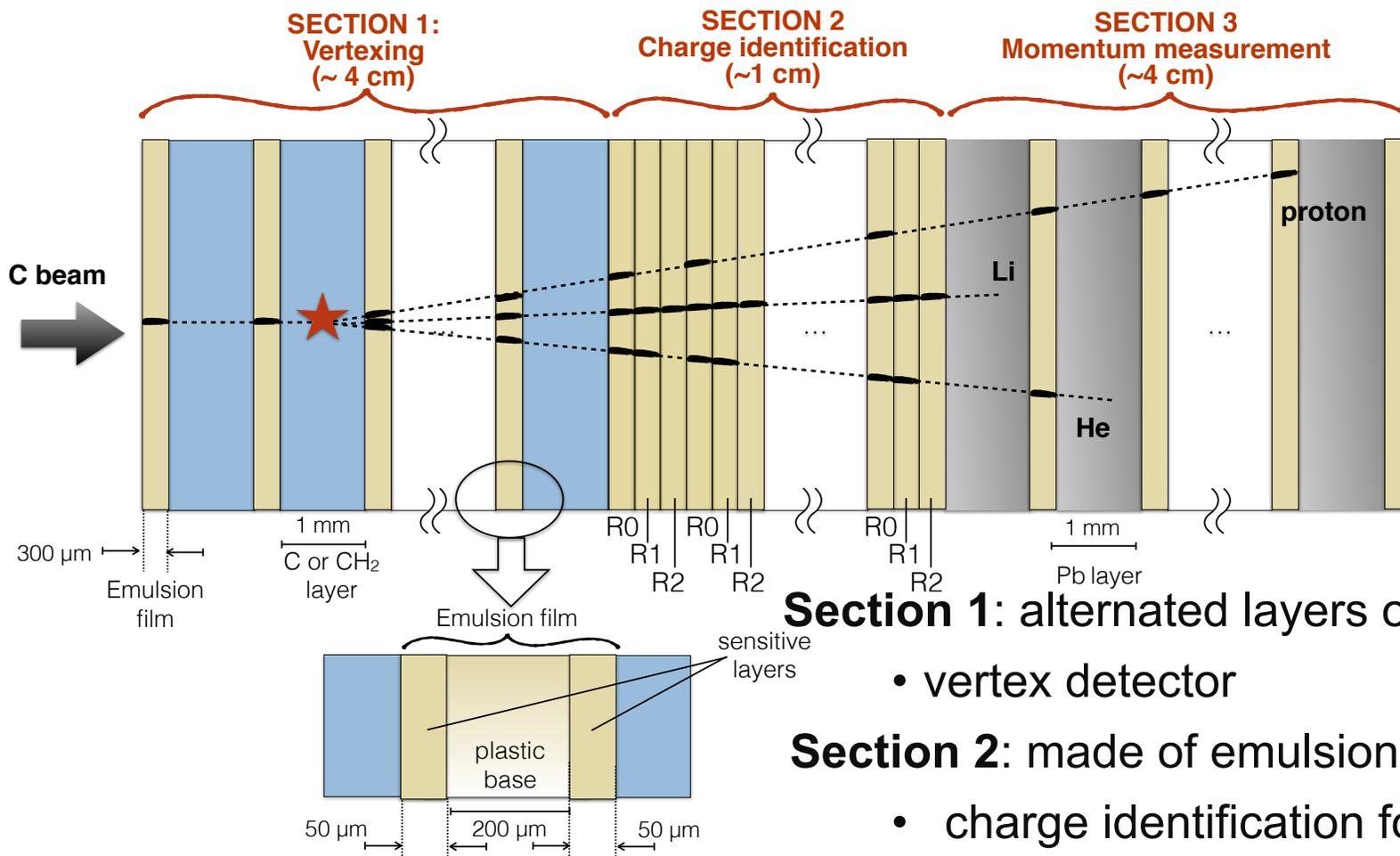
**Section 1:** alternated layers of emulsions and target (C/C<sub>2</sub>H<sub>4</sub>)
