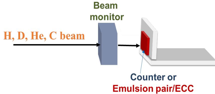
**Beam Monitor by the Perugia group:** silicon microstrip detector (strip pitch  $250\ \mu\text{m}$ , thickness  $350\ \mu\text{m}$ , total area  $8 \times 8\text{cm}^2$ )
