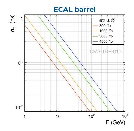
With proper attention to clock distribution, reduced shaping time, and high ADC sampling rates (160 MHz), can achieve ~ 30 ps time resolution for 30 GeV photons at high integrated luminosity (limited by S/N of existing APD photo-detectors)
