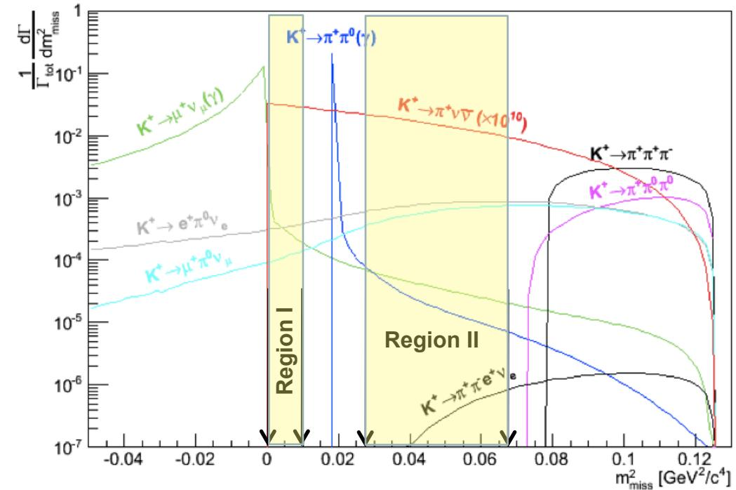
Background rejection relies on **Kinematics** ( $15 \text{ GeV}/c < P_\pi < 35 \text{ GeV}/c ; m_{\text{miss}}^2$ ) used in conjunction with **Particle ID, Veto systems** and **sub-ns timing**
