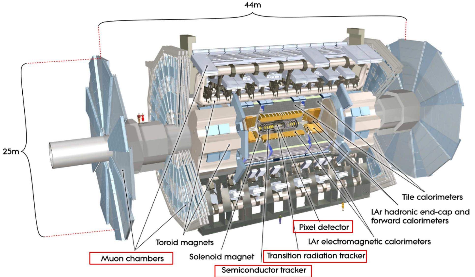
Inner detector and muon chambers most important for B physics
