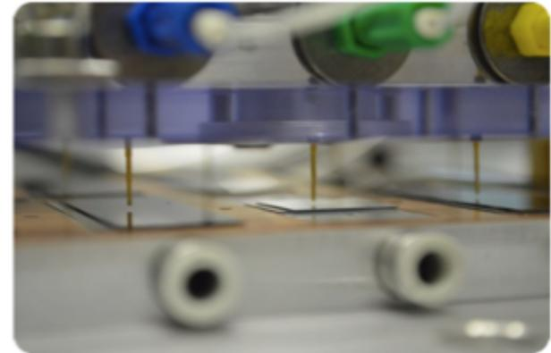
Sensors are bump bonded and automatically probed before vacuum testing to 1000V with spring loaded needle contacts to ASIC backplane
