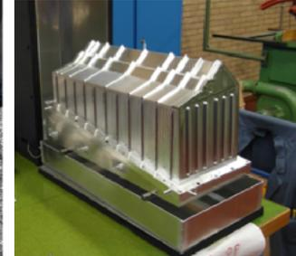
Internal mould support during machining steps
