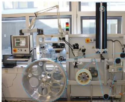
Custom winding machine using a threaded wheel
