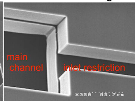
Two step channel etching
