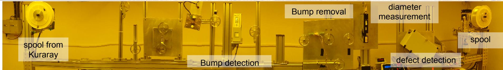
All fibre spools scanned for mechanical defects and irregularities (so far ~6000 km scanned).
