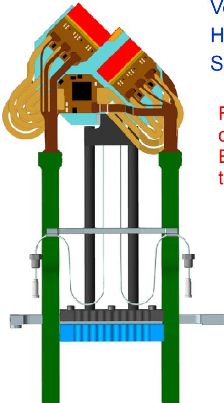
Four sensors per module (sensors on other side shown with dotted lines)
