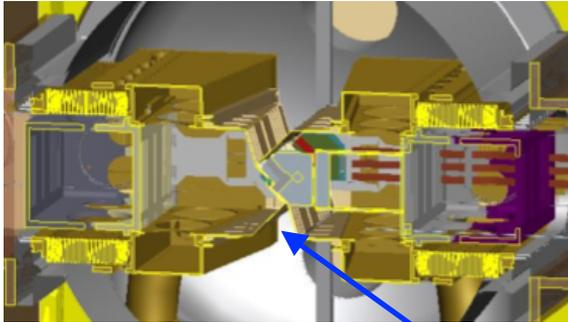
The VELO is separated from the primary vacuum by the 1.1 m long thin walled “RF foil” which also shields the detector and guides the beam wakefields
