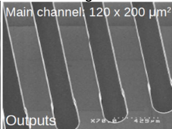
channels output directly to connector
