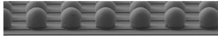
SEM image of  $55 \mu\text{m}$  pitch SgAn bumps
