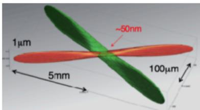
$$\text{luminosity: } \mathcal{L} = \frac{\gamma_{\pm}}{2e_e} \left( 1 + \frac{\sigma_y^*}{\sigma_x^*} \right) \frac{I_{\pm} \zeta_{y\pm}}{\beta_{y\pm}^*} \left( \frac{R_L}{R_{\zeta_y}} \right)$$
