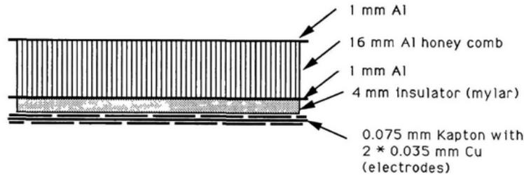
Insulator from a thin Mylar foil winded around many times using a highly resistive glue
