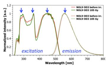
Radiation hardness tests on NOI 9 WLS: no irradiation effects on excitation/emission peaks up to 105 Gy
