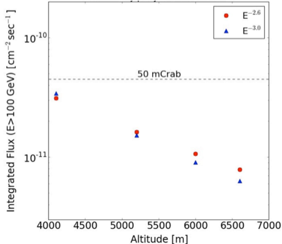
Sensitivity for one year of observation of an array of 900 tanks with 900 PMTs at different altitudes
