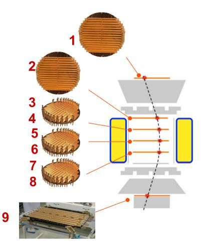
9 layers of double sided silicon microstrip detectors 192 ladders / 2598 sensors/ 200k readout channels
