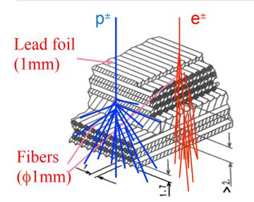
A precision, 3-D measurement of the directions and energies of gammas and electrons up to 1 TeV
