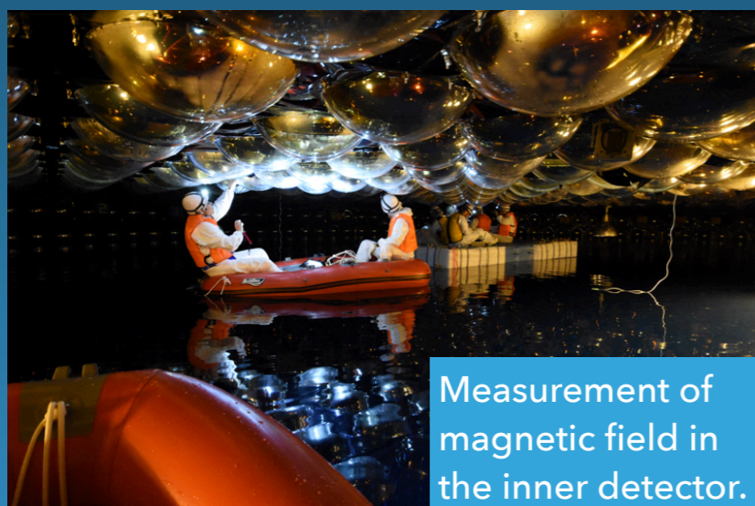
The water level is about 3m. The ID PMTs will be appeared to the surface of water soon..
