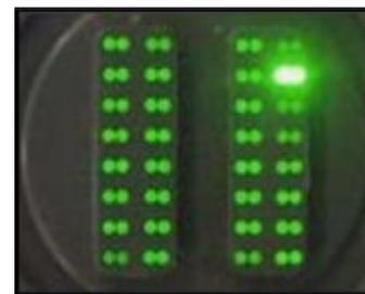
Instrumented with wavelength-shifting fibers and avalanche photodiodes
