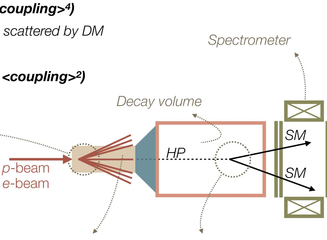
Long high Z target or collider Decay to SM particles
