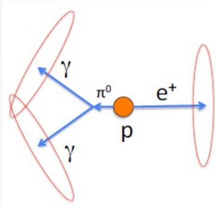
$e^+$  and photons are detected as e-like rings  $\rightarrow$  final state is fully reconstructed (practically background free)
