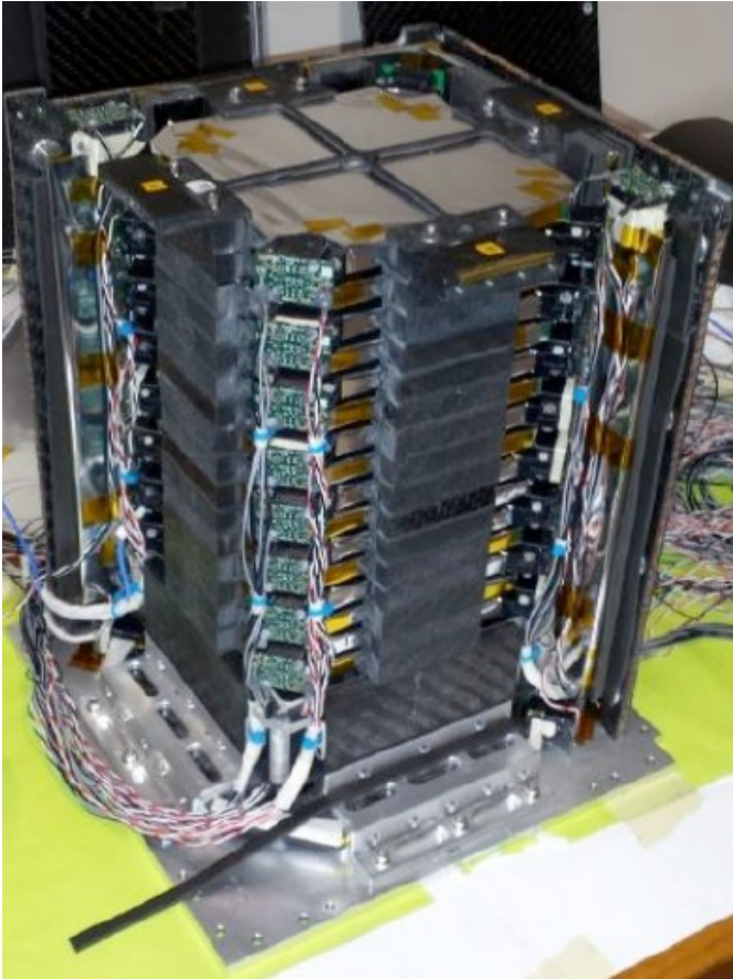
on the left the assembled scintillator tower
