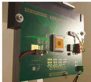
Study ongoing for the dose rate calibration with Si PIN diodes\_
