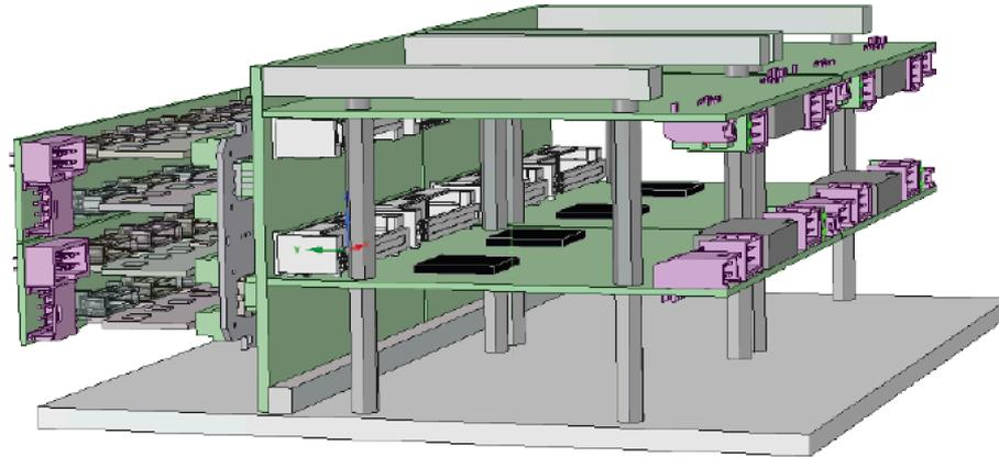
Automatic test setup under preparation, using the FEB + System Controller developed in Ferrara for FEB and Back-Boards QA to test 4 ECs, using the dark-box + LED illuminator concept developed in Edinburgh for Ma-PMT QA (with cooling system)
