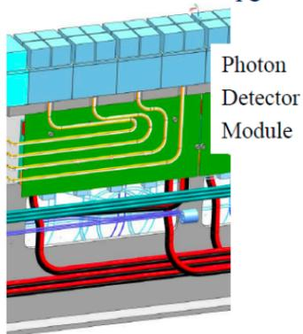
Photon Detector Module: 16 MaPMTs,
