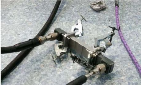
WR90 Waveguide Filter VNA Measurement vs HFSS
