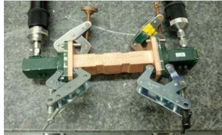
WR90 Waveguide Filter VNA Measurement vs HFSS
