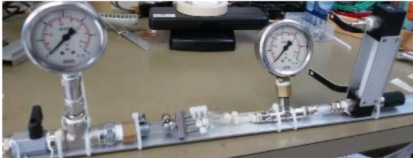
*Pressure drop measurements with compressed air (INFN Genova)*
