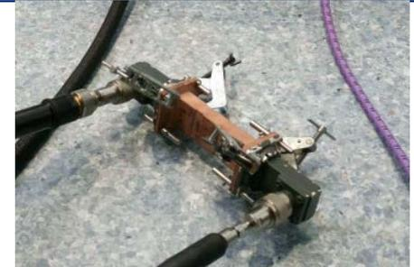
WR90 Waveguide Filter VNA Measurement vs HFSS
