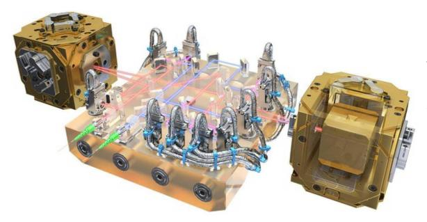
Test masses (TMs): cubes of 70% Pt-30% Au 4.6 cm side 2 kg mass 38 cm distance
