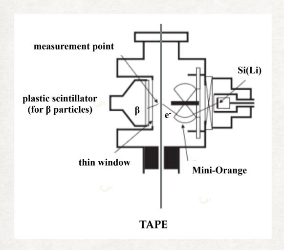
ICE spectra will be acquired in anticoincidence with the signals in the plastic scintillator in order to reduce the  $\beta$ - particle background emitted in the decay of the parent nucleus
