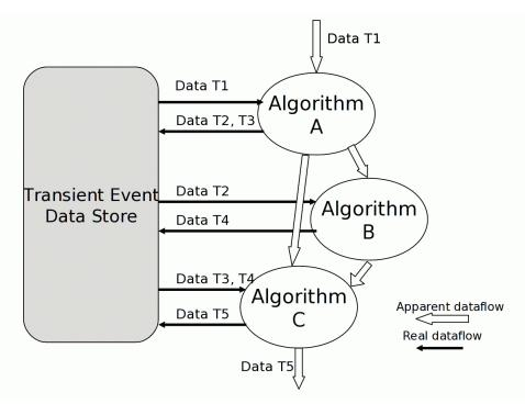
Highly configurable frameworks allow for a specific choice of modules (sequences, etc.) to be run via simple edits to a python config script, without needing to relink a full binary. A standard stub application reads the config script and loads the necessary shared libraries as dynamic "plugins"
