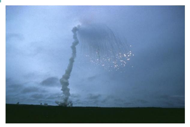
First Ariane 5 flight, destroyed just after launch as it veered out-of-control, along with a \$400M scientific mission (Cluster).
