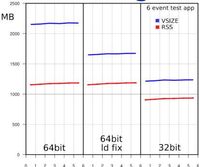
CMS example: with a custom linker script, ~500MB can be removed by relinking the numerous and very small libs (see plot). Another ~100MB would be possible from linking external libs in the same way. (Workaround to keep systems using VSIZE happy for now...)
