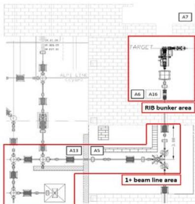
Fig. 1. The SPES RIB bunker area (room A6), the 1+ beam line area (rooms A5 and A13) and the service rooms A7 and A16 (located upstairs with respect to the other rooms represented in this figure).
