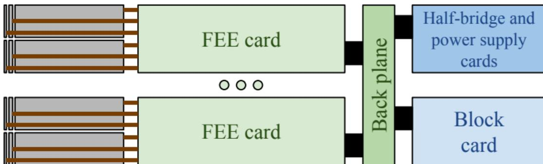
*8 FEE cards are connected to a block card via a back plane.*
