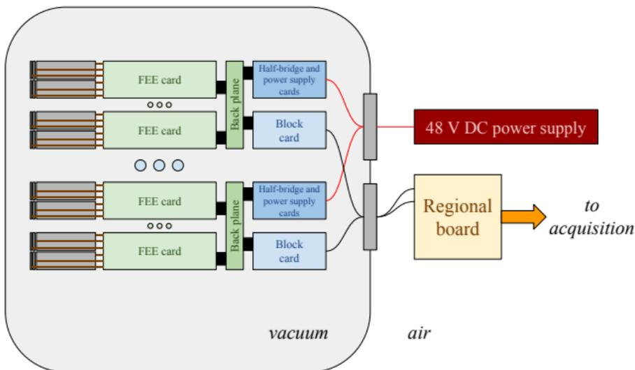
*up to 36 block cards are connected to a regional board via a full duplex 3 Gb/s optical link*
