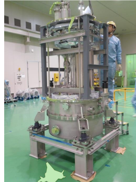
After sealing cavity, assembly of major parts in ISO class-7 clean room
