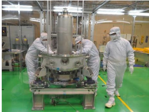
Sealing operation of cavity in ISO class-1 clean room
