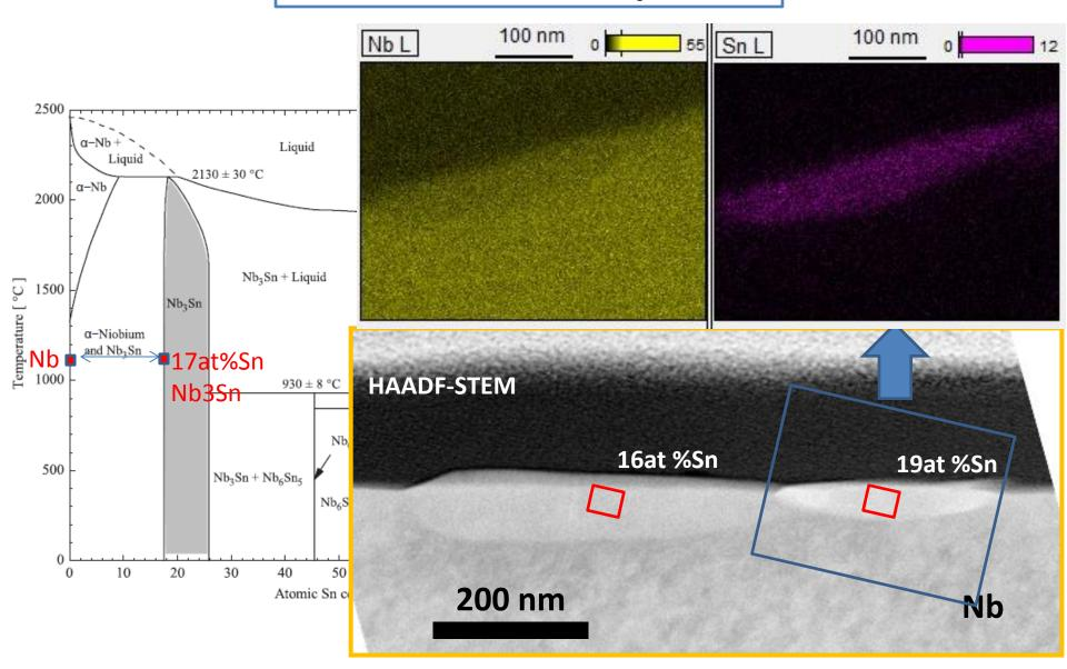
STEM-EDS implies that nucleated Nb<sub>3</sub>Sn grain have low Sn-composition  $\rightarrow$  It agrees to the phase diagram: low Sn-Nb<sub>3</sub>Sn and Nb at Nb<sub>3</sub>Sn/Nb interface.
