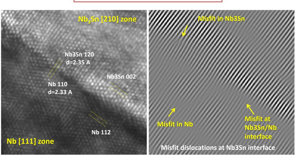
Semicoherent interface between Nb<sub>3</sub>Sn and Nb
