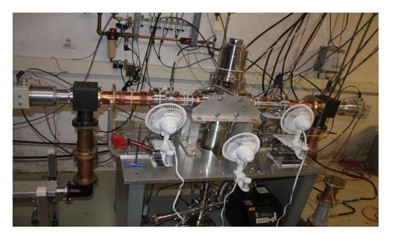
Pair of couplers were successfully tested up to 30 kW, CW, full reflection, 90 dgr. step reflection phase.
