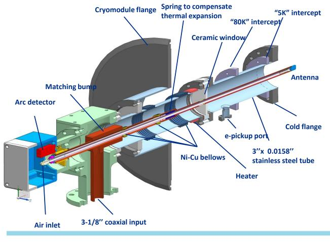
Antenna: Copper 0.5", air cooled, HV bias.
